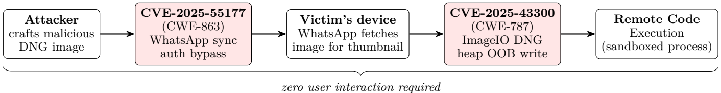
Fig. 1. End-to-end flow of the 2025 zero-click chain. Red nodes mark the two patched CVEs. Only the victim’s phone number is required; no action by the victim is needed for the chain to reach code execution.
